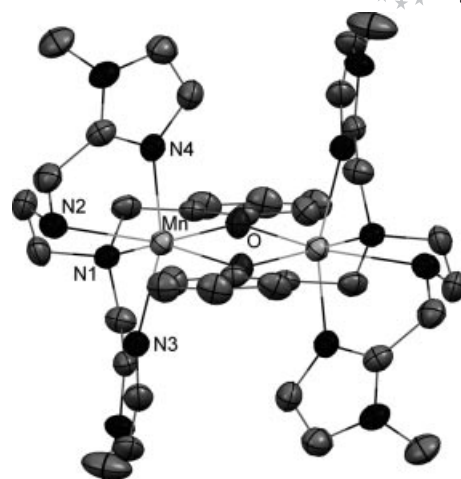
Figure 1. Ellipsoid plot of the centrosymmetric cationic moiety 1 , produced with Mercury 1.4.2. [56] Ellipsoids are drawn at 50% probability level. PF 6 − and H atoms have been omitted for clarity.
